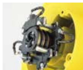
Compact 30, 35 or 75 amp modular collector rings can accommodate up to 16 conductors. All brushes are spring loaded copper/graphite for positive electrical contact.
