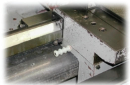
Shown: Application photo illustrates small envelope size required of the Enidine One-Shot Emergency Stop Shock Absorber.
