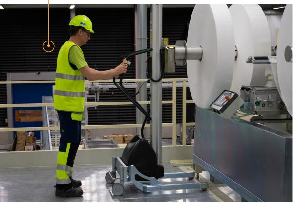
At SCA in Sweden, several lifting trolleys are used to pick up reels from pallets and transport them to machines. The reels are easily positioned and mounted on the machines. All with the ergonomic help of TAWI lifters.
