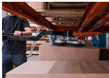
A vacuum lifter on an articulating arm enables you to reach far into pallet racks.
