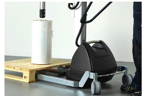
On several models, the measurements of the wheels make it possible to drive the lifter into a pallet in three different ways.
