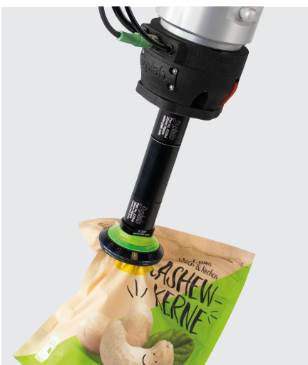
Adapter plate with 3/8" female, extantion and MX cup handling a bag with nuts
