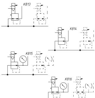
K814 = MANIFOLD reg., NO relieving, electrical command, and external servo pilot supply K815 = MANIFOLD reg., relieving, electrical command, built-in pressure gauge and external servo pilot supply K816 = MANIFOLD reg., NO relieving, electrical command, built-in pressure gauge and external servo pilot supply
