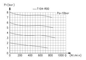
Flow diagram for model: T108-R00 Pa = Inlet pressure (bar) Pr = Regulated pressure (bar) Q = Flow (Nl/min) Flow diagram for model: T104-R00 Pa = Inlet pressure (bar) Pr = Regulated pressure (bar) Q = Flow (Nl/min)
