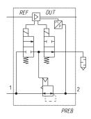
Version with integrated exhaust valve and internal servo-pilot supply
