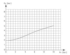
This diagram shows the relation between working pressure (Px) and pilot pressure required in order to operate the valve (Py). The opening pressure of the unidirectional valve is 0,3 bar.
