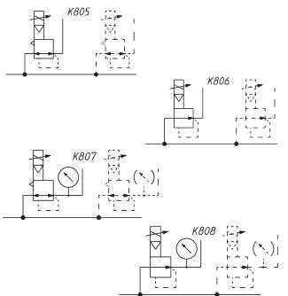
K805 = MANIFOLD reg., relieving, electrical command K806 = MANIFOLD reg., NO relieving, electrical command K807 = MANIFOLD reg., relieving, electrical command and built-in pressure gauge K808 = MANIFOLD reg., NO relieving, electrical command
