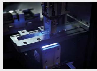
UV Black light provides evidence of eventual traces of hydrocarbons, grease or particulate.
