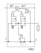
3 ways N.C. version with internal servo-pilot supply
