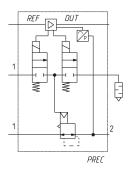
3 ways N.C. version with external servo-pilot supply
